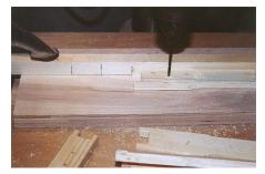
Begin by drilling 1/8" diameter holes centered in the end bars. 5 holes are drilled on 9-1/8" (deep) end bars, evenly spaced. 3 holes are drilled on 6-5/8" (medium) end bars, evenly spaced. A simple jig is made by using a scrap piece of wood and making marks on it that equate to the spacing of the holes to be drilled.
