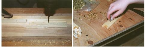
Once the holes are drilled, install brass eyelets into the holes. A setting tool can be purchased.
