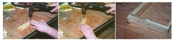
To install the wire, start by setting a small headed nail just above the top eyelet on one side of the frame.
